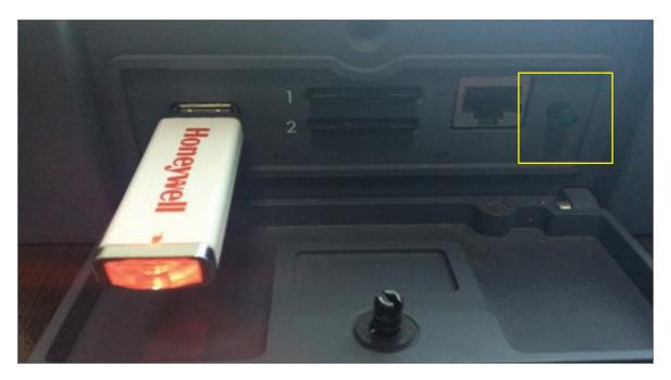
**NOTE**: During the load process, both lights will flash amber. When both the lights turn green; it indicates that the configuration loading is successful. If the left light flashes and the right light is steady amber, it indicated that the configuration has failed. The ADG100 will write a status file to the USB with the file name install\_tailnumber.log.
